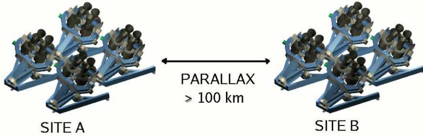
**Fig. 1.** Configuration of final system, able to cover whole Swift’s field of view. The parallax will allow to automatically reject short optical flashes from near Earth objects in real time.
