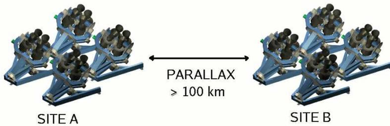
Fig. 1. Schematic view of the final "Pi of the Sky" detector.
