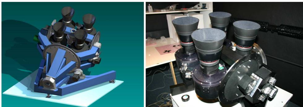
**Figure 1:** Robotic mount - scheme and the final construction.
