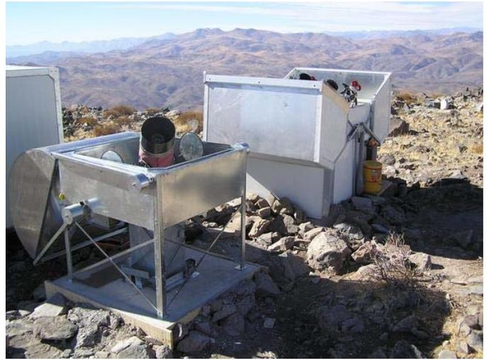
Fig. 7. The ASAS 10” telescope, which could be used to follow up “ $\pi$  of the Sky” triggers.
