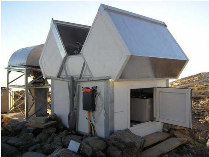
Fig. 5. The ASAS / “ $\pi$  of the Sky” dome, partially opened. A PC controlling the system seen through the service door.
